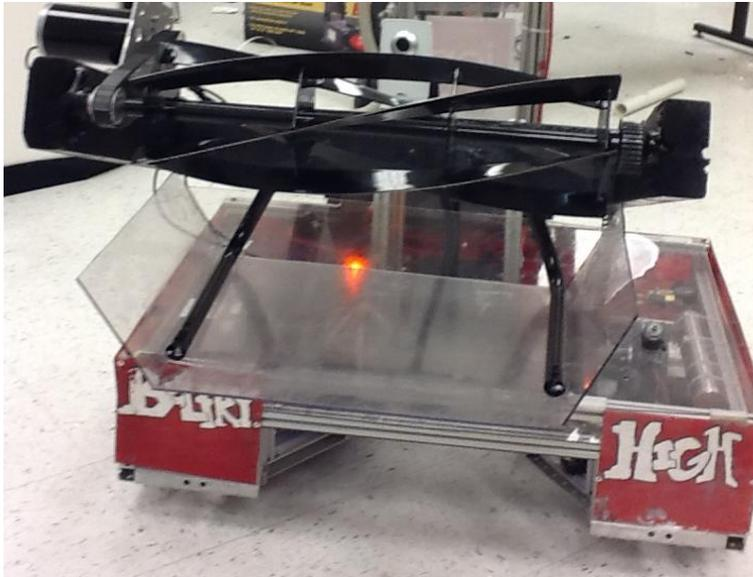
The main motor used was a CIM motor. This standard motor powered the continuous miner and also the wheels for driving the unit within the mine. A camera, also mounted on the mining arm, allowed the operator to see where and how to move the RMV.
